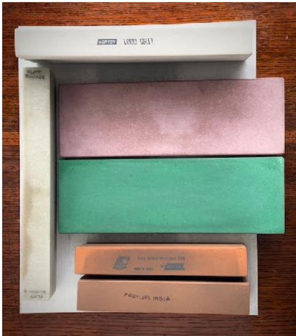
Stones can be roughly shaped with a belt grinder, always using water or oil as a cutting fluid. It is easy to overheat the stone, causing fractures, so grinding should be done very slowly. Stones will also ruin the belt within a few minutes.
