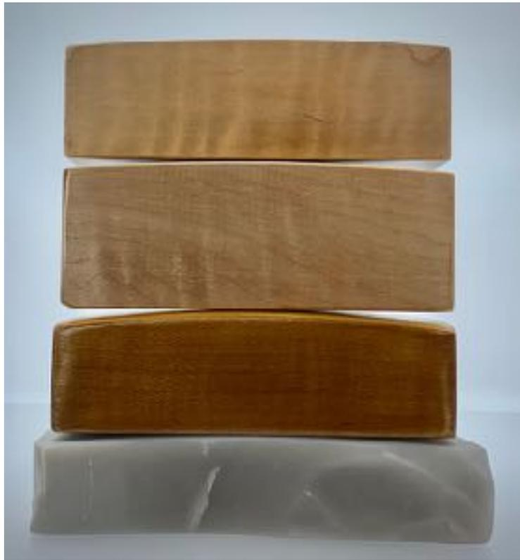
This image shows a progression of 6.5' elliptically surfaced razor honing stones, starting with an India Fine, Hard Arkansas, Jadeite for ripping off the burr, Blue-Black or White Translucent Arkansas for polishing, and finally a Jende diamond pasted stropp for the keen toothy edge. Mineral oil, with a drop of oud for scent, is used as the cutting fluid for all the stones.
