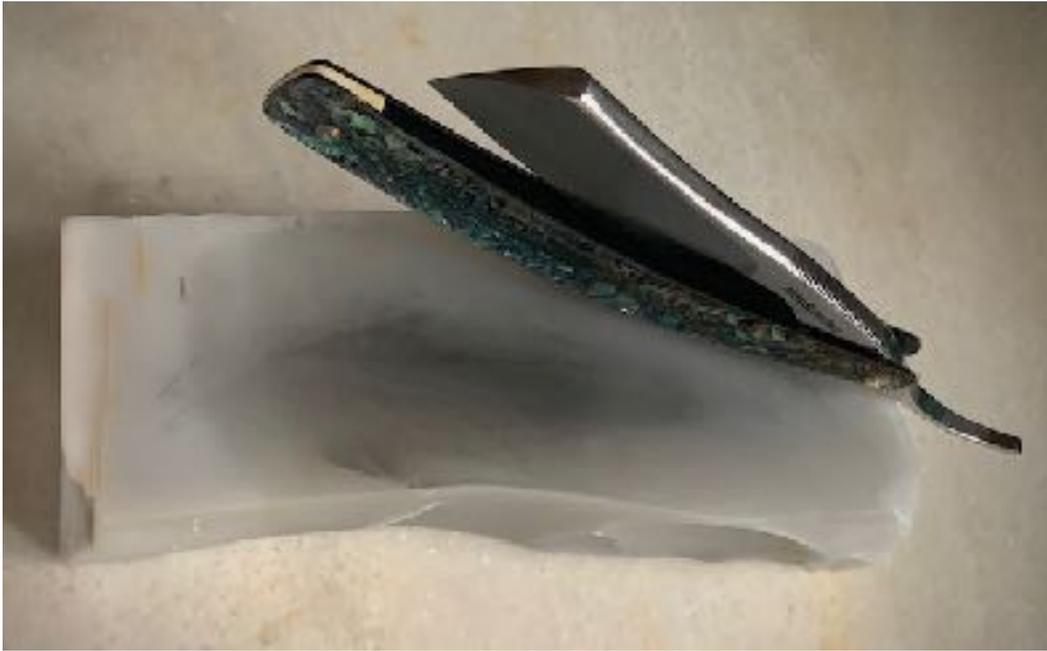
The thin, concave bevel created by the convex elliptical surface makes a keen edge for a close and pain-free shave.
