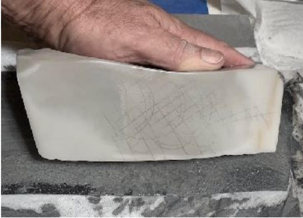
It takes several hours of grinding on 36-grit abrasive paper to shape the stone into the elliptical form. Making maple wood blocks with an elliptical surface is much easier. Adhesive-backed abrasive paper, or film, can be applied to the wood blocks to make a convex sharpening surface for knives.
